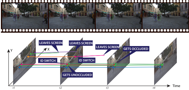
Figure 4: Detection Errors – Scene from the MOT2016 dataset
